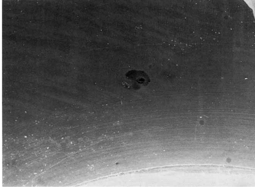
Figure 13 Contact path at magnification ( \times 20 ). Polyacetal cup. Velocity: 400 rpm. Load on the contact: 160 N. Dry conditions.
