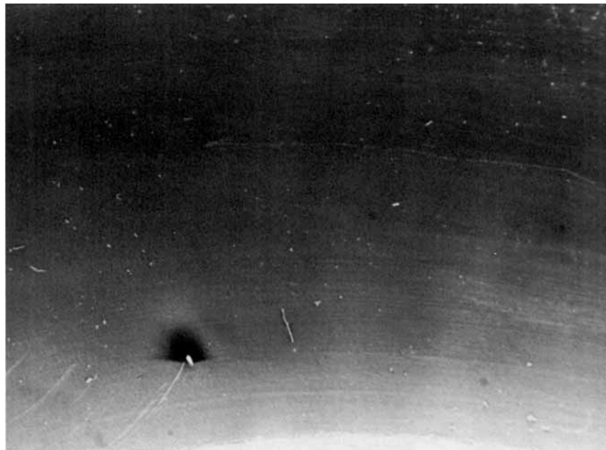
Figure 7 Section of the contact path at magnification ( \times 12 ). Nylon 6.6 cup. Velocity: 400 rpm. Load on the contact: 120 N. Dry conditions.
