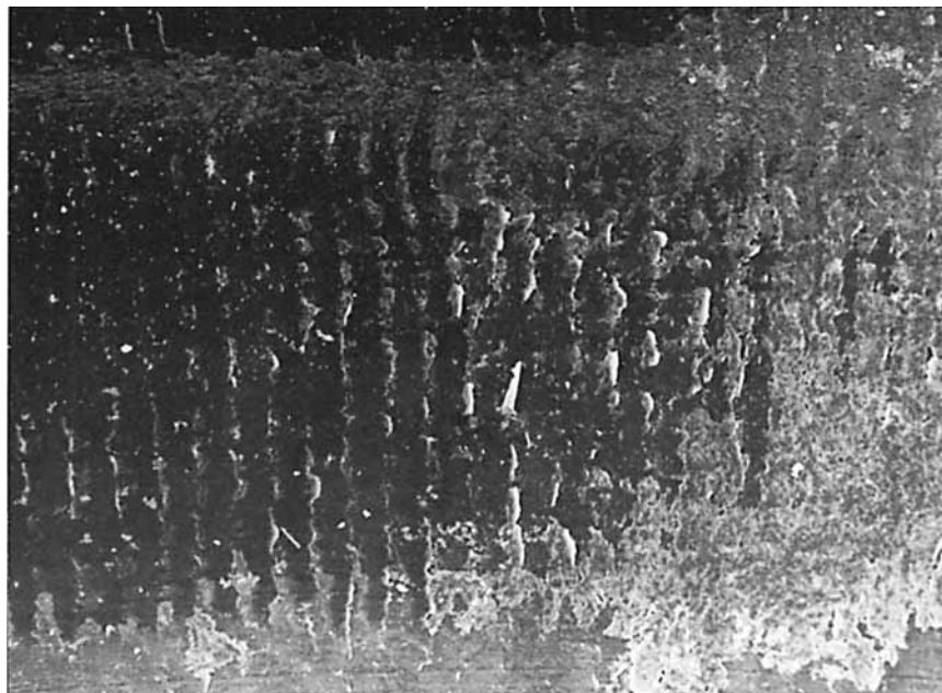
Figure 4 Trailing edge of reattached polymer at magnification ( \times 50 ). Remaining data as in Fig. 3 legend.
